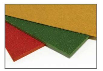
Fiberplate<sup>®</sup> is manufactured by building up multiple layers of fiberglass reinforcement and specially-formulated resins. The result of this process is a solid composite panel offering both bidirectional strength and corrosion resistance.
