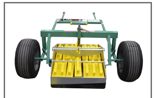
To move cart, position cart, raise DynaWeight, and move to new location.
